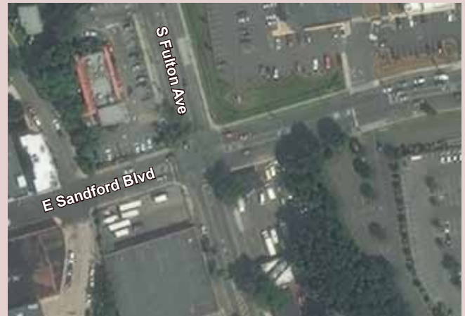
Existing conditions at this intersection include buildings placed in deep parking lots with little building frontage along the streets. Sidewalks are narrow and have few street trees and lights.
