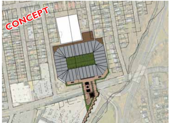
Option A Site Plan: An enclosed field, surrounded by two tiers of seating, a parking structure and a plaza that spans East Sandford Boulevard.
