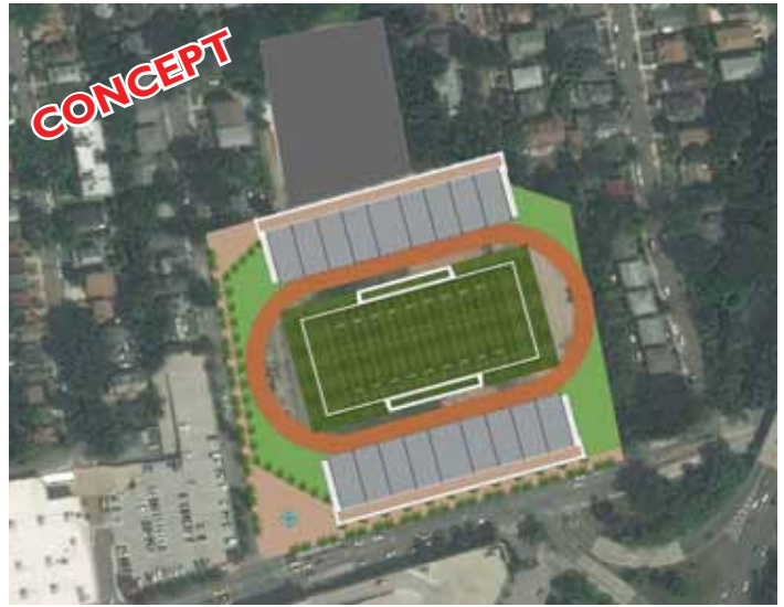
Option B Site Plan: A field with seating on either side of the field and a competition track.
