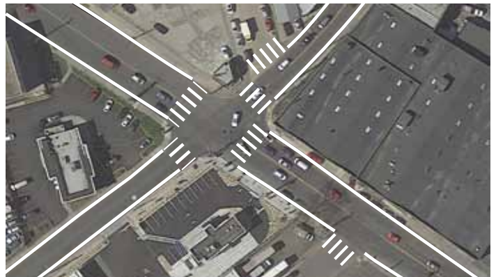
This concept shows Columbus Avenue with striped bike lanes. Fulton Avenue also has striped bike lanes, buffered using on-street parking, or raising the bike lanes up to the level of the curb. This is possible because the width of the Fulton Avenue right-of-way is greater than that of Columbus Avenue.
