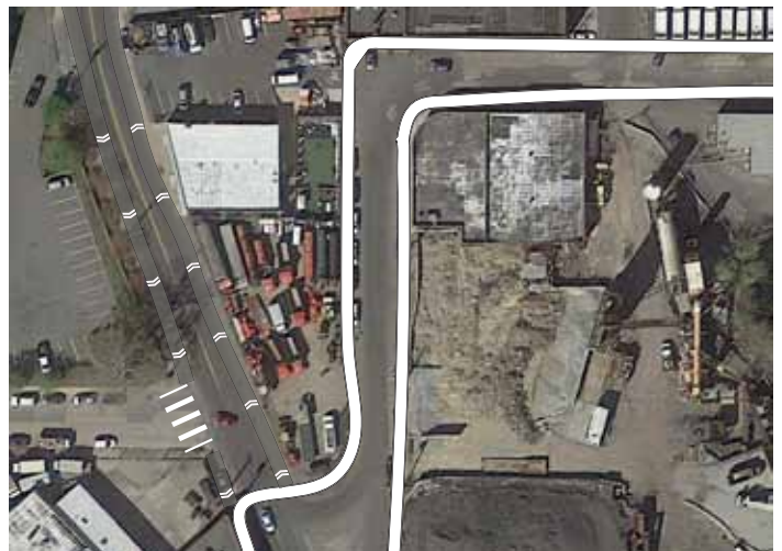
The Canal Street and Columbus Avenue intersection is composed of striped bike lanes on both sides of Canal Street. For Columbus: striped bike lanes south of Canal Street, but north of Canal Street stripped bikes and automotive traffic share the lane with “sharrows.”
