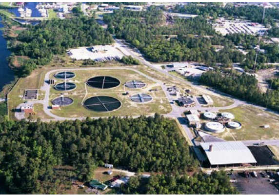
Southside Wastewater Treatment Plant The Southside Wastewater Treatment Plant was put into service in 1972 as a 6,000,000-gallon per day treatment facility. It was later expanded and the capacity increased to 12,000,000-gallon per day to serve New Hanover County and the Town of Wrightsville Beach.
